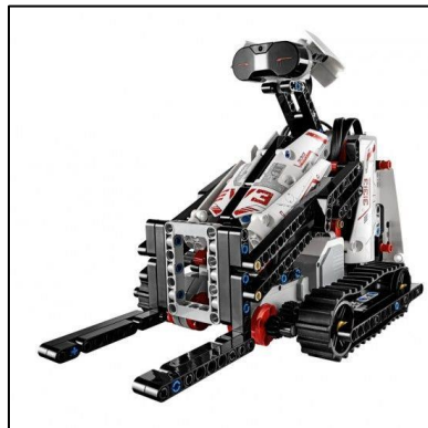
Figure 2: The Lego Mindstorms EV3 Forklift
